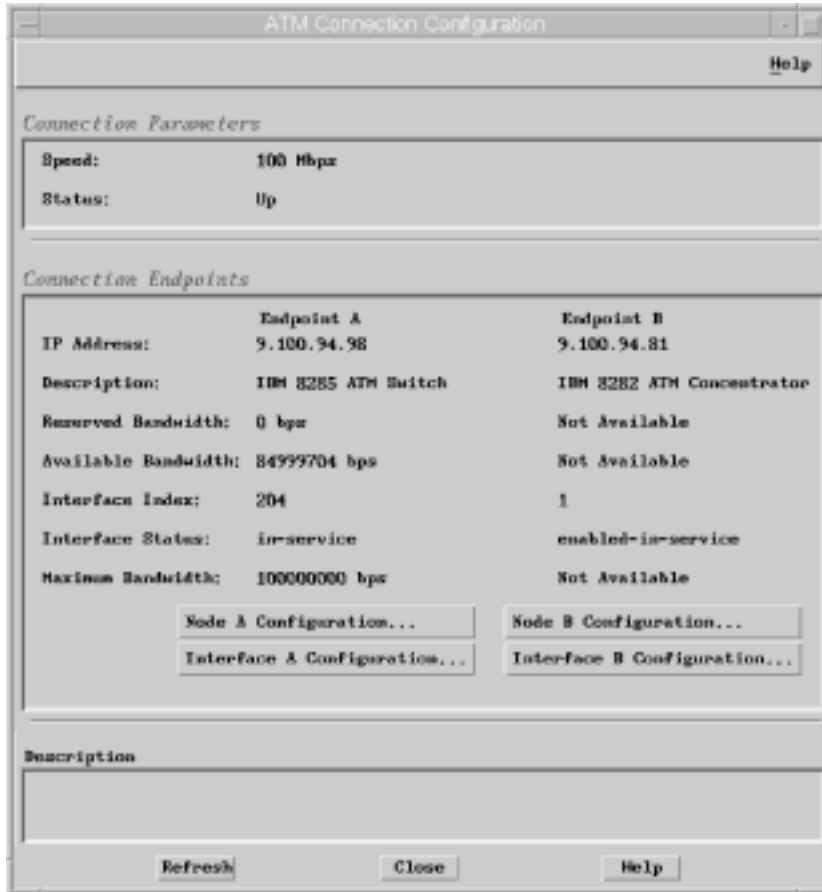
Figure 31. ATM Connection Configuration Panel
