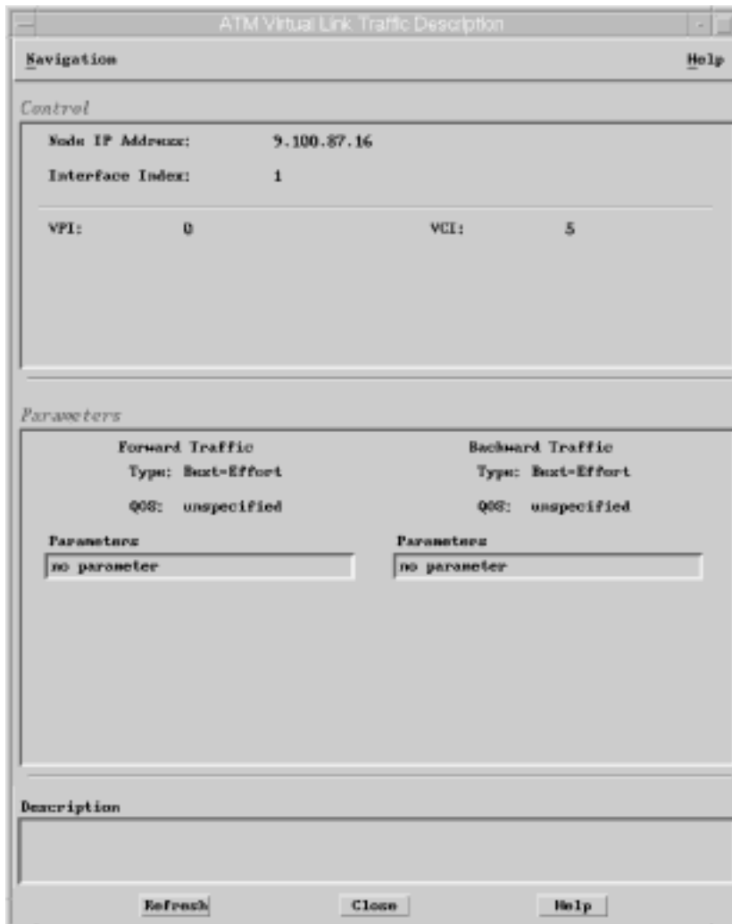
Figure 45. Virtual Links Traffic Description Panel
